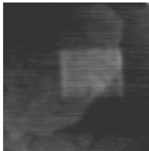
Figure 7. AFM image ( 300 \text{ nm} \times 300 \text{ nm} ) depicting the relative heights for a \text{CF}_3 -terminated SAM (the light colored square) nanografted into a \text{CH}_3 -terminated SAM. The darker color corresponds to a lower height. The height differences between the nanografted patterns and the matrix are about 0.2 \text{ nm} but ranges over several images from near zero to 0.2 \text{ nm} . The image clearly shows that the grafted pattern follows the surface features of the gold step.
