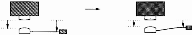
Fig. 2. Method of force measurement. Mechanisms used to change the reference separation are calibrated at large surface separation, where no forces are present.
